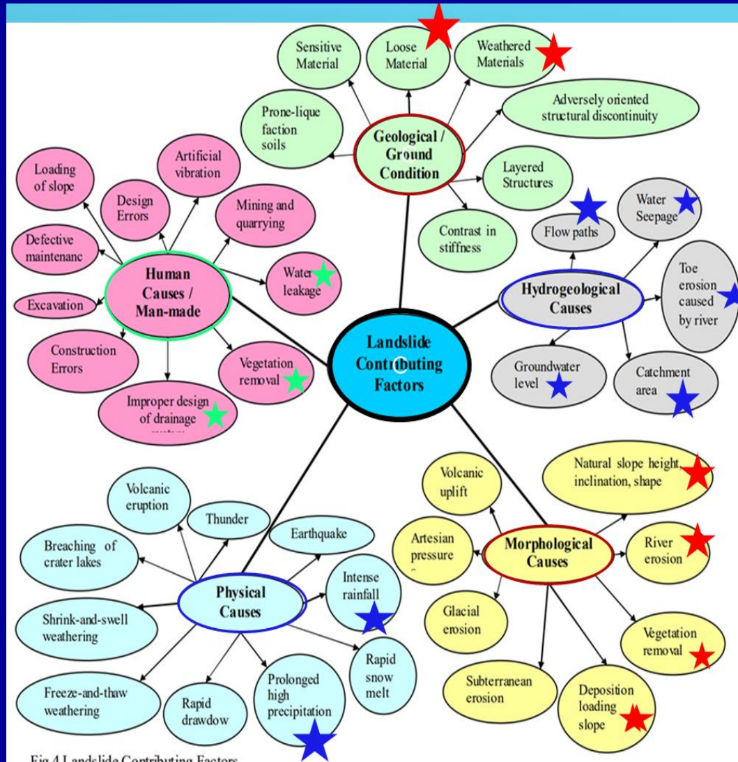
Fig.4 Landslide Contributing Factors
